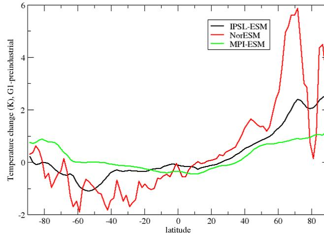
**Figure 2: Zonal mean surface temperature anomaly in experiment G1 (4xCO<sub>2</sub> balanced by reduced solar constant) relative to a preindustrial control simulation. Results of IPSL-ESM (black) and MPI-ESM (green) are averaged over 50 years, NORESM results (red) over 10 years. Note: In the graphs for IPSL-ESM and NorESM a temperature bias has been removed that was resulting from an inexact balancing of the radiative forcing.**
